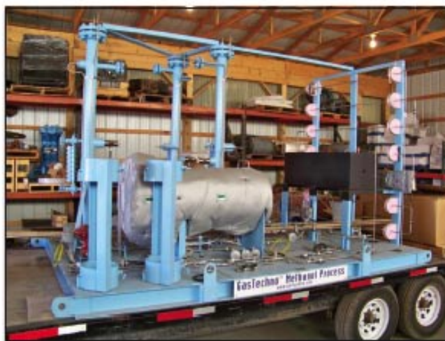
GasTechno Process converts methane into methanol.
